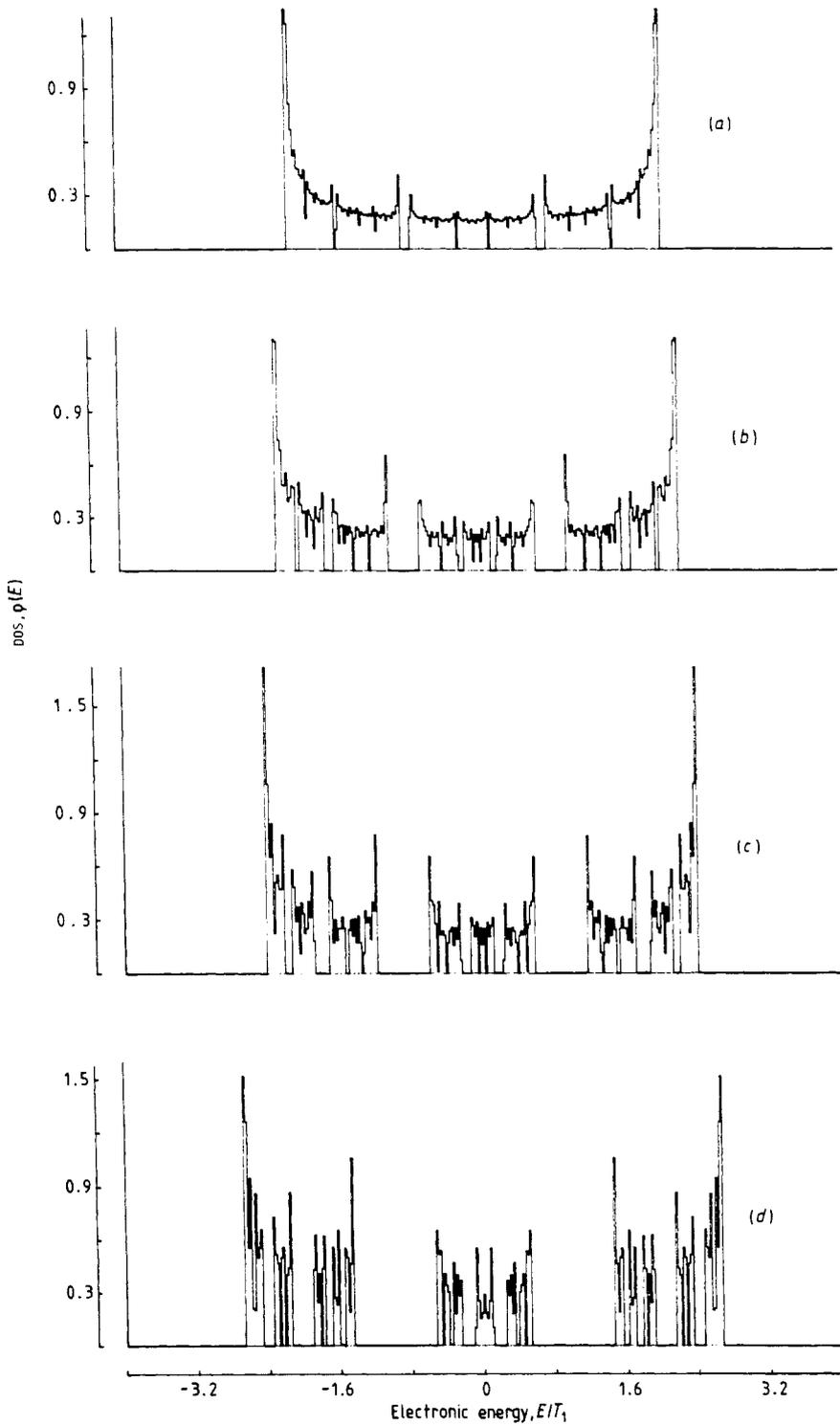
**Figure 3.** The electronic DOS of a one-dimensional Fibonacci quasi-crystal for the symmetrical case:  $\epsilon_1 = \epsilon_2 = 0$ .  $T_1 = 1$ .  $T_2 =$  (a) 1.1, (b) 1.3, (c) 1.5, (d) 1.8.
