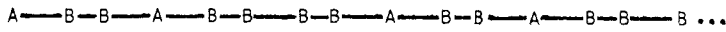
Figure 1. A schematic representation of a one-dimensional Fibonacci quasi-crystal. A and B signify possible different atomic levels.
